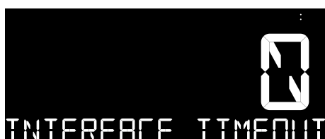
Fig. 30: Connection monitoring deactivated
